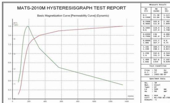
Magnetization curve (Permeability curve)
